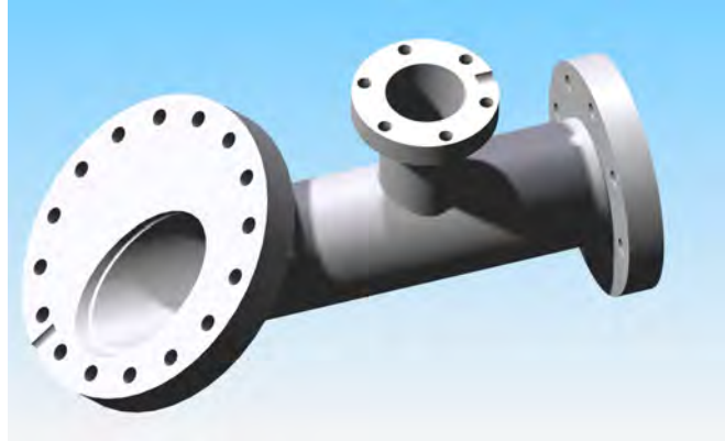
Figure 4.6: End section of the dumping section, with port for the TMP angled at 45^\circ to maximize pumping efficiency.
